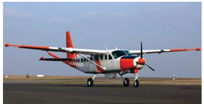
Three cesium magnetometer horizontal gradiometer system installed on a CESSNA C208B GRAND CARAVAN AIRCRAFT in wingtip pods and a tail-boom (stinger).
