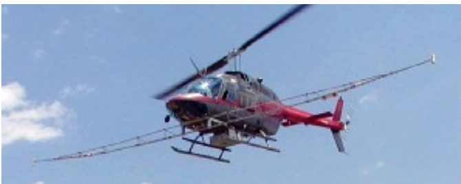
Two cesium magnetometer horizontal gradiometer system installed on a rigid-boom mounted on a BELL 206L3 JET RANGER HELICOPTER .
