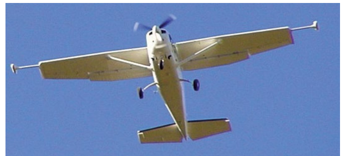
Two cesium magnetometer horizontal gradiometer system installed on a CESSNA C206 AIRCRAFT in wingtip pods.
