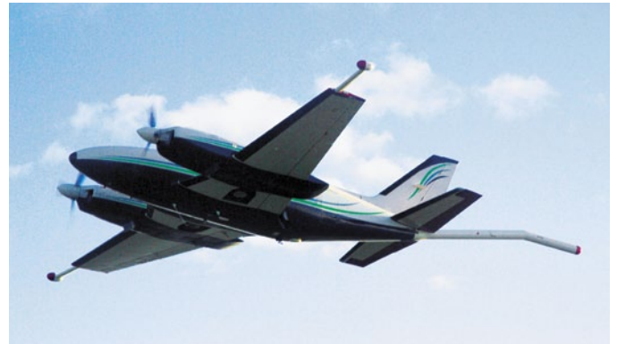
Three cesium magnetometer horizontal gradiometer system installed on a PIPER PA-31 NAVAJO AIRCRAFT in wingtip pods and a tail-boom (stinger).
