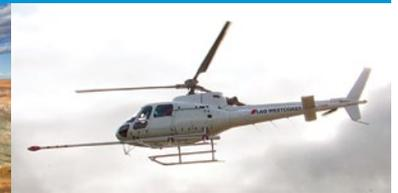
The objective of surveying with a multi-channel, gamma-ray spectrometer system and a large volume gamma-ray sensor is to detect subtle characteristic radiation patterns as indicators of subsurface hydrocarbon accumulations over petroliferous terrain. ISMAP and **GAMMASENSE** techniques may be applied independently of each other, however, it is practical and cost effective to combine them in one multi-sensor, multi-method survey.
