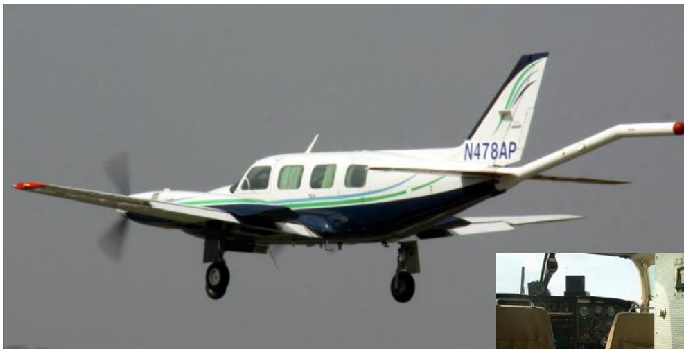
*Piper PA-31 Navajo Survey Aircraft in ISMAP/GammaSense configuration*
