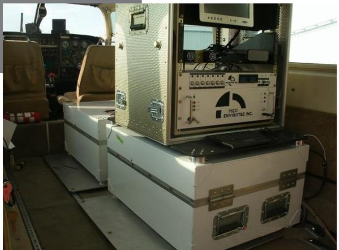
*GammaSense detector packages installed in the cabin of a Piper PA-31 Navajo survey aircraft*
