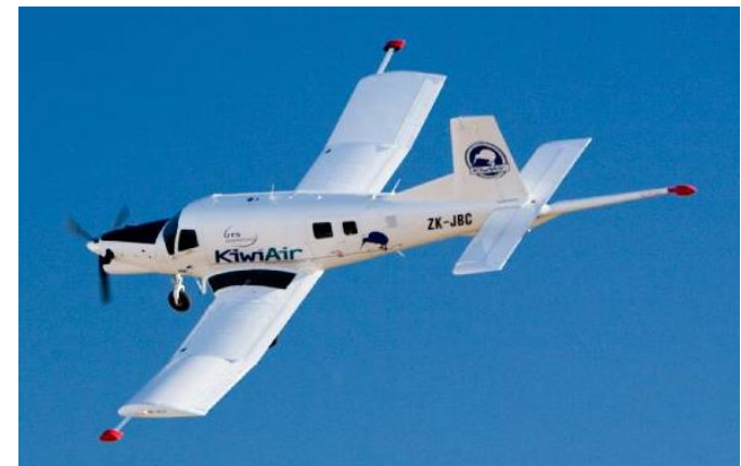
3-sensor magnetometer installation on a PAC-750XSTOL AIRCRAFT
