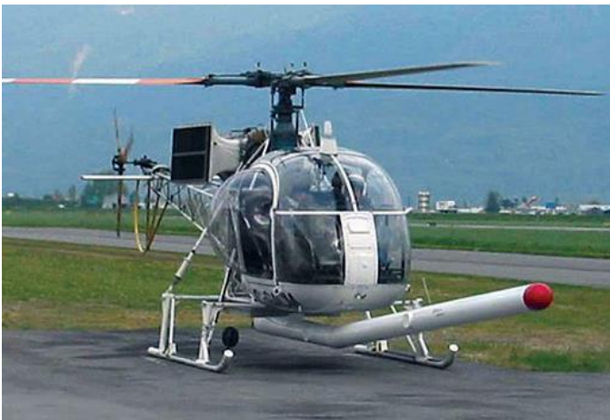
High-resolution magnetometer aerofoil installed on a EUROCOPTER AS315B LAMA HELICOPTER
