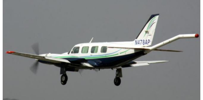
Magnetometer installation on a PIPER PA-31 NAVAJO AIRCRAFT
