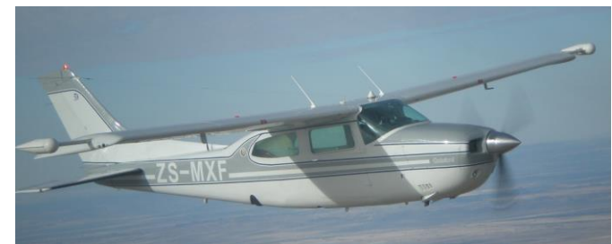
2-sensor Magnetometer installation on a CESSNA C210 AIRCRAFT
