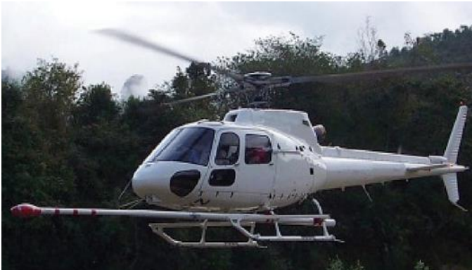
Total-field magnetometer installation in a rigid-boom on an EUROCOPTER AS350B2 A-STAR HELICOPTER
