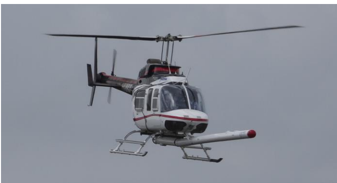
High-resolution magnetometer aerofoil installed on a BELL 206B3 JET RANGER HELICOPTER
