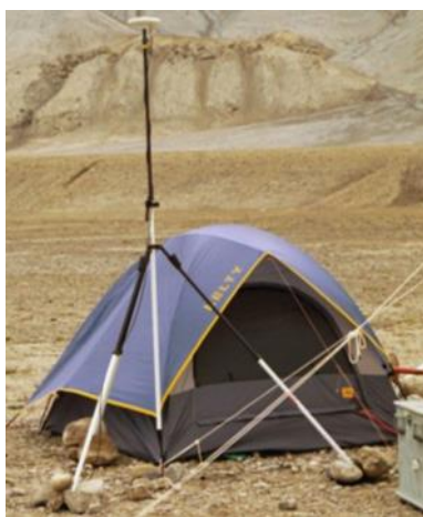
GPS Base Station
