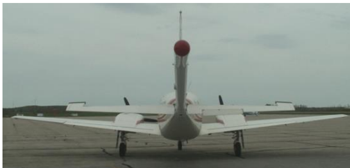
The rigid-boom stinger for the high-sensitivity cesium magnetometer on a Piper PA-31 Navajo aircraft
