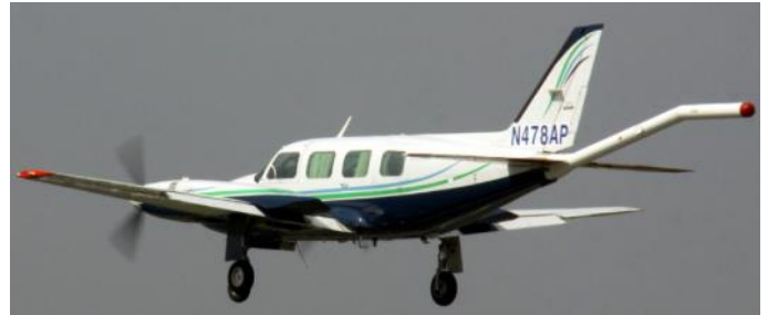
Piper PA-31 Navajo twin-engine survey aircraft - equipped with an airborne Gravity Meter, high-sensitivity magnetometer in a tail-stinger
