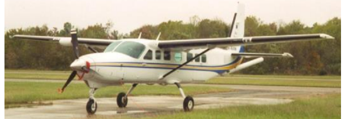
Cessna C208B Grand Caravan turbine engine survey aircraft - equipped with TAGS-6 Gravity Meter, high-sensitivity magnetometer in tail-stinger
