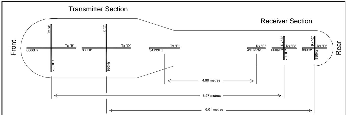
Layout and dimensions of the transmitter and receiver coils in the HUMMINGBIRD EM sensor
