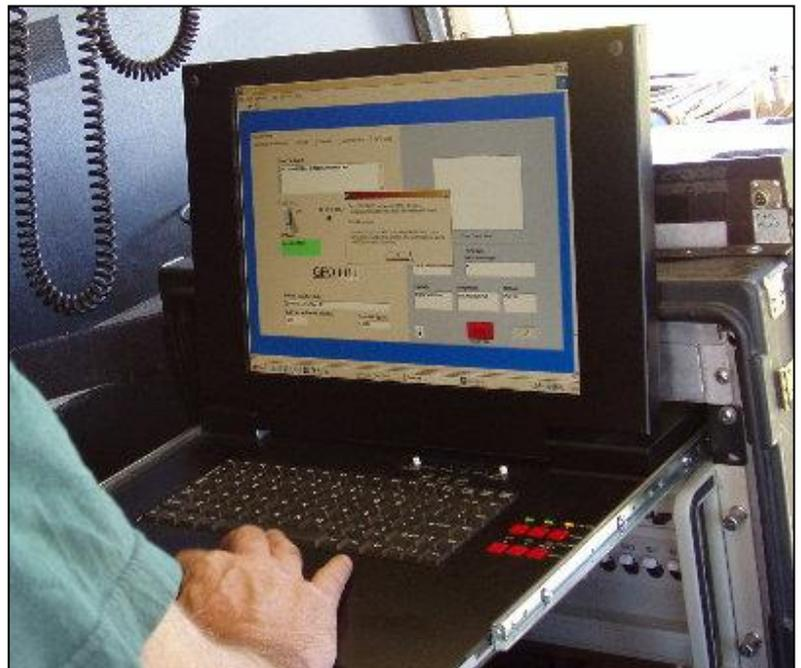
*Operator's screen/keyboard assembly – HUMMINGBIRD EM system*
