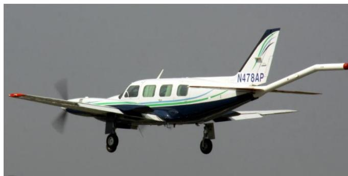
*Piper PA-31 Navajo aircraft with magnetometer tail-stinger*
