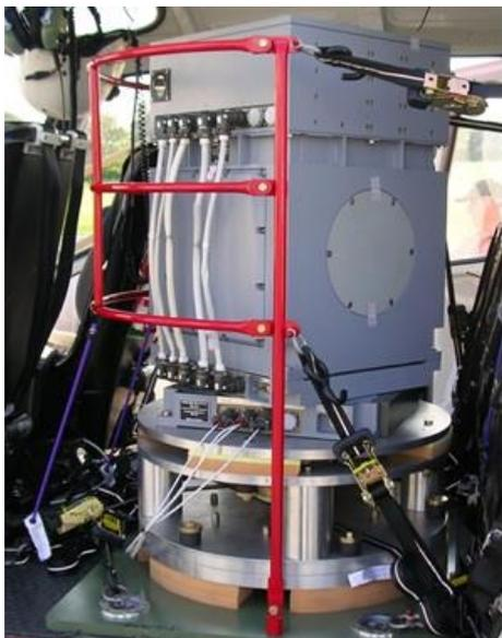
*GT-2A Airborne Gravity Meter installed on aircraft*
