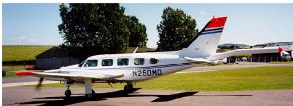
Figure 5 – Piper PA-31 Navajo survey aircraft. This aircraft is equipped with long-range fuel tanks and has a flight duration in excess of 7 hours
