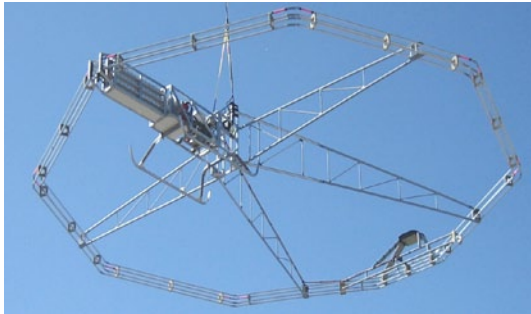
THEM Multi-Sensor time domain EM Magnetic System.
