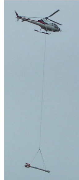
Hummingbird 5-frequency EM/MAG System.
